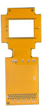
Model NO:PCB02457 Base Material:PI (Polymide) Certification:RoHS, CCC, ISO Transport Package:Vacuum Packed Specification:L1, 1 OZ copper, FPC, 0.12mm, no stiffer, yellow coverlay Trademark:FasTechCircuit Origin:Mainland China Production Capacity: 1000000 PCS/monthly
